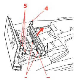
**6.** Rotate the rollers forward with your finger and repeat step 5 until the rollers are clean.
